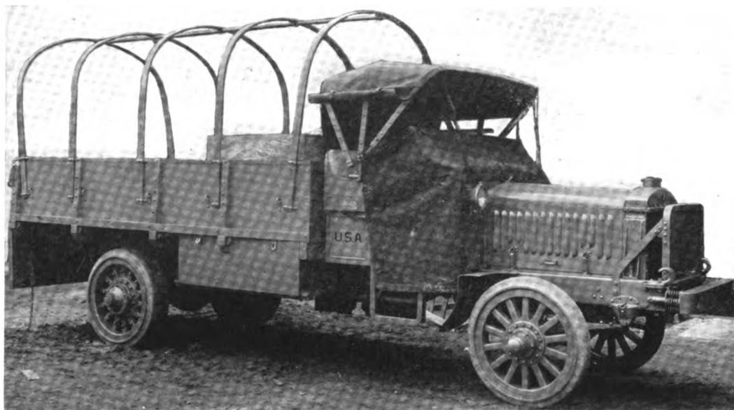
Class B War Truck, Designed and Produced by the Automobile Industry, Rated at 6,000 Pounds Load Capacity, with Standard Service Body
